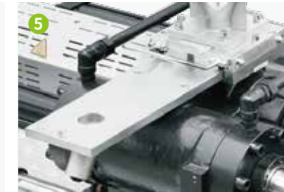
5 人性化設計：移動料斗滑軌 (320T 及以下) User-friendly design: movable hopper rails (60T-320T)
