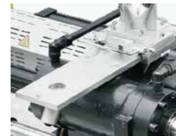
Movable hopper guide rails(standard feature for 90T-320T)
